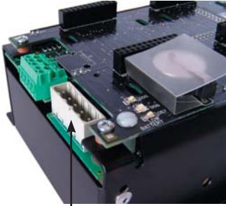
Removable DeviceNet Connector
